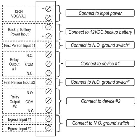
The First Person Input function suspends the operation of the PT Series annual timer. If a relay is turned on before the first man feature is activated, the relay will remain on until the first man feature is deactivated.
